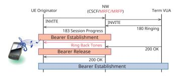
Alert-Info: Provides substitute ring back tone using Alert-Info, one of the Early Media switching function
