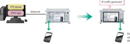
For the transmission and reception of the UE, use iPerf application which is widely used for throughput testing.
